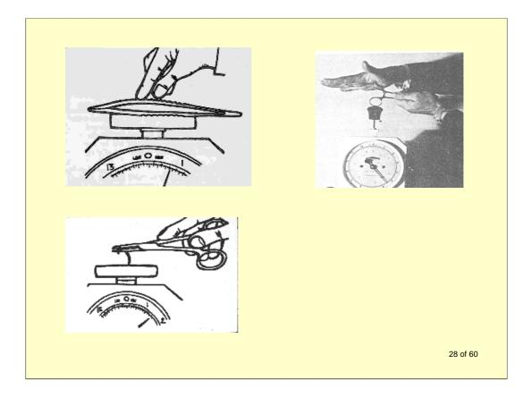
The upper left picture shows measurement of the stiffness of dissecting forceps (one arm looks too curved, please ignore). Force is applied at the usual fingertip position until the tips of the instrument touch.
