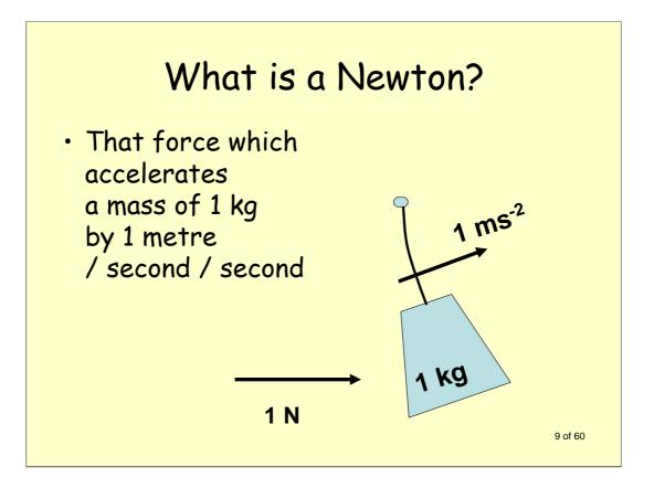
Here's my attempt at a diagram to illustrate the definition through the idea of pushing on a pendulum.
