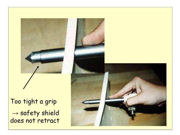
However there are a few traps. At ECRI (the world's largest biomedical consulting group) scientists showed how a tight hand grip on the trocar and cannula stopped the safety mechaism allowing the point to spring back inside the cannula once the skin had been penetrated. The persisting point could cause severe and even lethal damage during the inisial setting up for laparoscopic surgery.
