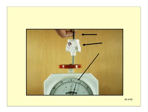
One of the problems was loss of sense of tocuh because of friction between instruments and the cannulas they were slid through. It was easy to measure this friction by the simple arrangement shown – a port resting on the scale, and an instrument pushed downwards through it. This might take several N, results I never recorded formally or published then.
